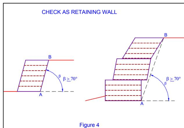
In this analysis, the gabion support works are considered to be a monolithic structure.
