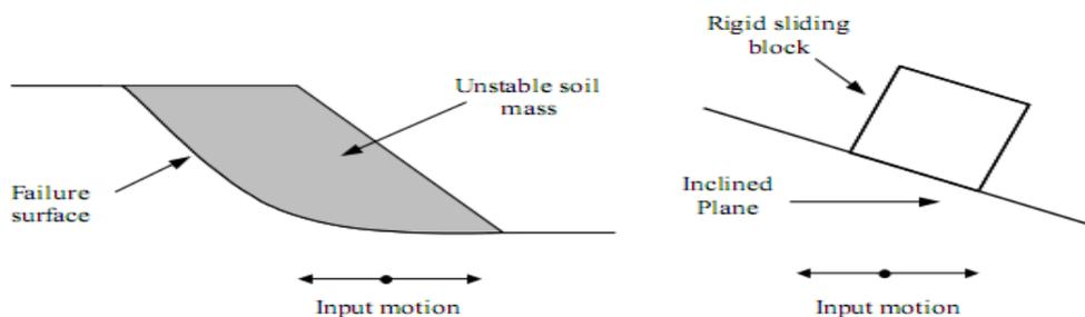
Figure 5.1 Analogy between potentially unstable slope and a rigid block on an inclined plane
