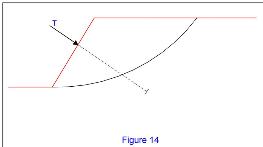
In this case the program will operate a distribution of the load with an angle of  $90^\circ$  with respect to the direction of the reinforcing units (for a total of  $180^\circ$ ) using the same procedure adopted for the linear loads.
