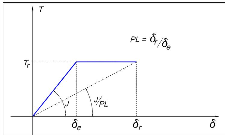
$T_r$  = conventional unit breakage force (kN/m)
