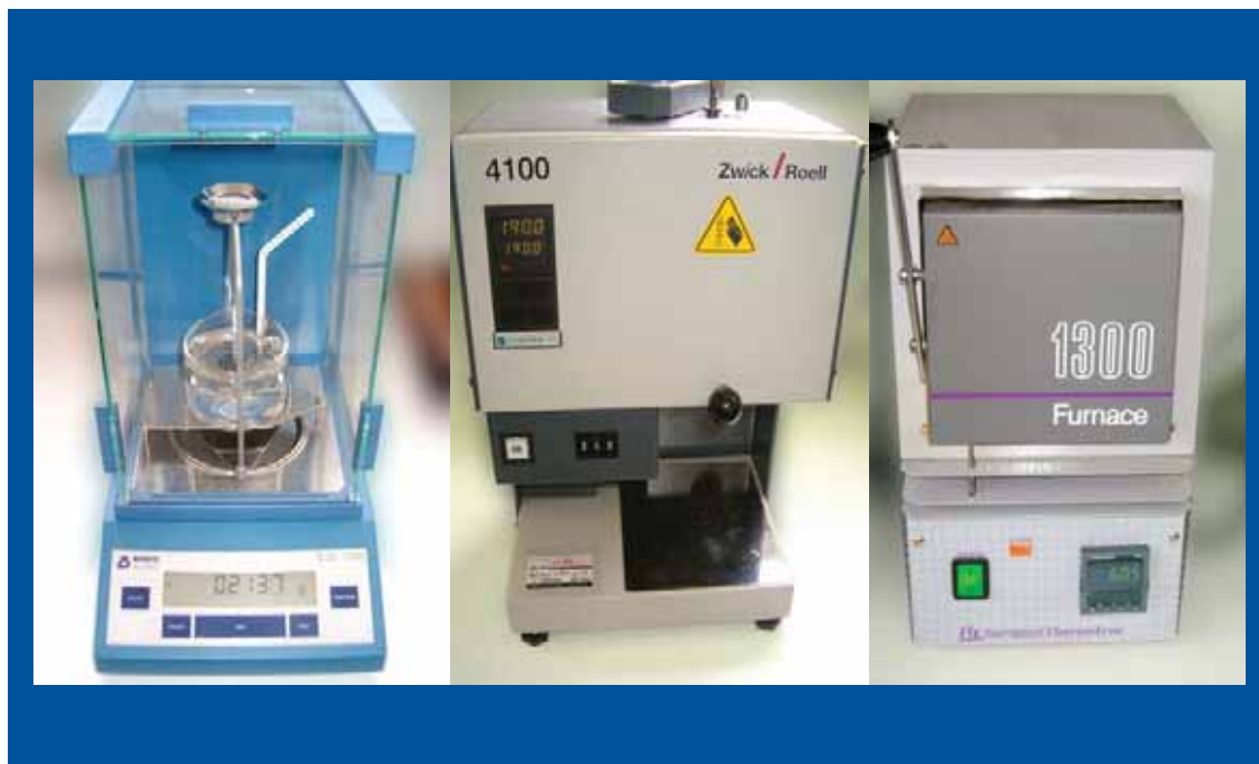
From left to right: Density, Melt Flow Index and Carbon Black Content. ◀ ◀ ◀ ◀ ◀
