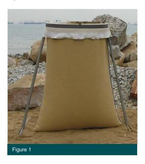
The ELCOROCK® Filling Frames are intended for suspending 0.75m³ ELCOROCK® containers while being filled with sand by excavators.
