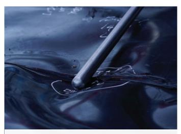
**ELECTRICAL INSPECTION** Electrical spark testing of the primary liner using bidim C
