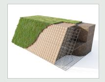
It is constructed using durable double-twist steel wire mesh, that forms an inclined front face Reinforced Soil Slope (RSS) with an integrated tail section for long-term structural stability. To encourage vegetation growth and improve erosion resistance, the facing is
