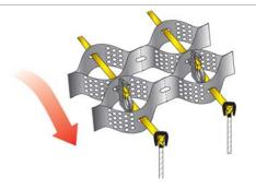
Figure 12 End Anchorage of Tendons
