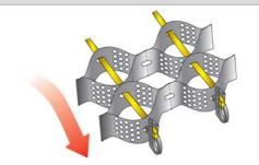
Figure 11 Termination of Integral Tendons
