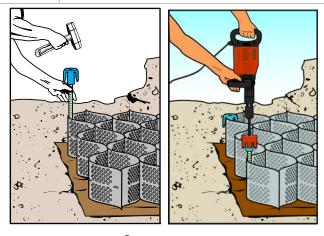
Figure 5 ATRA® Anchor Installation Methods
