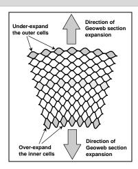
Figure 7 Tapered Expansion of Section
