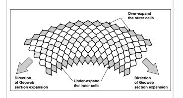
Figure 8 Curved Expansion of Section
