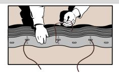
**Figure 10 Tendon Insertion**
