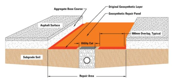
Image 6. Typical Utility Cut Geosynthetic Repair Detail (NTS)
