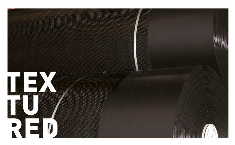
Atarfil offers two types of textured products, one with an asperity height of 0.9mm that can be described as the highest frictional performance on the market, and another with a 0.6mm roughness for applications which due to length of the inclined plane, gradient to traverse or support conditions do not require the maximum friction coefficient to be obtained while always maintaining a significant level thereof, as it could not be otherwise for such applications.
