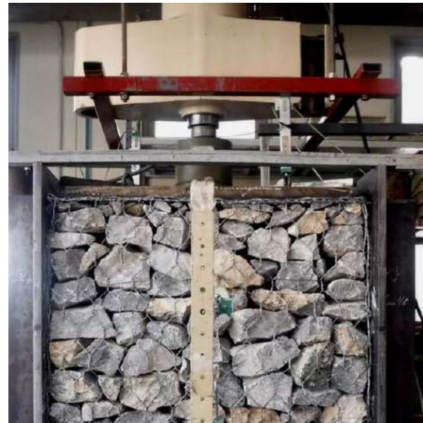
Full Scale Compressive Test
